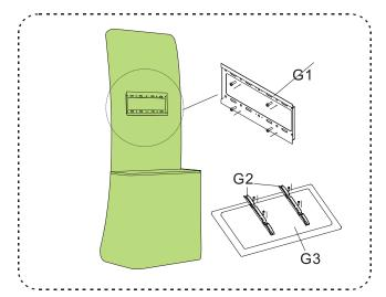
5.To use screws to fix the monitor holder frame onto the stand then install the upright bar on the back of monitor
