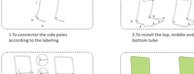
3.To install middle cross bar and the bottom upright tubes
