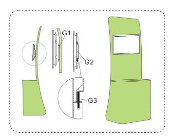
6. Afterwards put whole monitor onto the stand and fasten by using screw #G3
