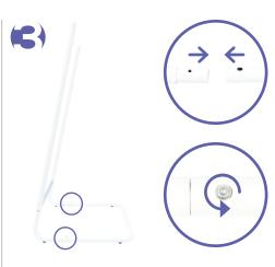
Connect the Bottom Tube and the bottom Leg Tubes to align holes together. Insert the screws and tighten to secure with allen key.
